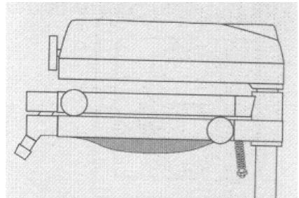
7.- LEAVE THE HEATER AND SUCTION CONNECTED DURING 10-15SG, UNTIL THE ADAPTATION IS COMPETED.
