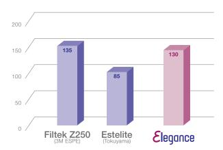
\* Source Spident R&D center internal data. International test standards - ISO 4049 : 2009; 7.11. Flexural strength measuring instrument. Universal testing machine.
